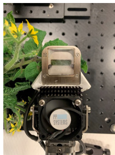
Figure 1. Leaf cuvette of the CIRAS-3
