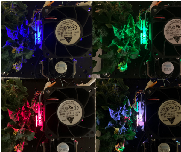
Figure 2. Different lights on in the TIGER Cub. The TIGER Cub is designed to mount directly to the leaf cuvette and consists of a single TIGER module with a re-configured LED array to accommodate the small window of the CIRAS-3 cuvette.
