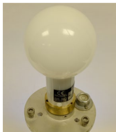
Figure 2: Spherical quantum sensor attached to a leveling plate. The diameter of the globe is 6.1 cm (2.4 inches). The sensor measures the amount of incoming photosynthetically active radiation (400-700 nm) from (almost) all directions (note that the stem of the sensor obstructs (some portion of the) light coming from below the sensor).
