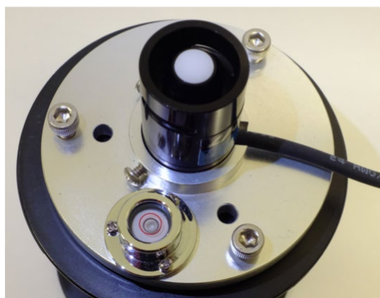
Figure 1: Regular quantum sensor attached to a leveling plate. The diameter of the sensor body (black) is 2.36 cm (0.93 inches). The sensor measures the amount of incoming photosynthetically active radiation (400-700 nm) from the hemisphere (dome) that extends upward from the horizontal plane at which the (top of the) sensor is placed.
