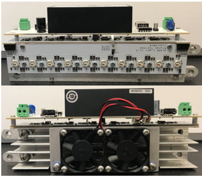
Figure 2: Two views of the TIGER light module. TOP – lighting side of the module showing 10 LED packages, each with 6 separate LEDs. The large black box on top is the AC/DC converter. BOTTOM – view of the module top showing cooling fans, as each module can dissipate up to 60 W at full brightness.
